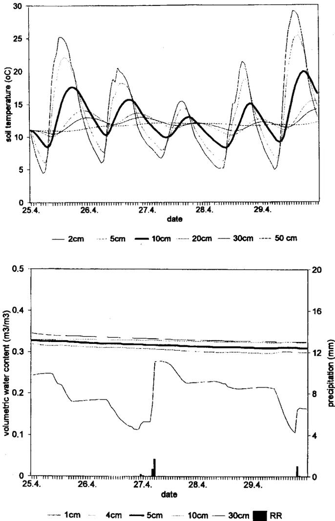
Figure 3: Hourly values of the soil temperature (top) and the soil volumetric water content (bottom) in different soil depths, computed with MEBIT for the period from 25<sup>th</sup> to 29<sup>th</sup> April 1991, in Bilje.
