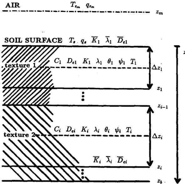
Figure 1: The arrangement of the variables in the model space used by space integration in MEBIT. The variables are denoted as in the text.
