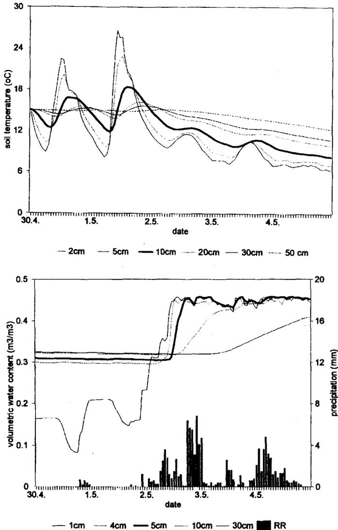
Figure 4: Hourly values of the soil temperature (top) and the soil volumetric water content (bottom) in different soil depths, computed with MEBIT for the time period from 30<sup>th</sup> April to 4<sup>th</sup> May 1991, in Bilje.
