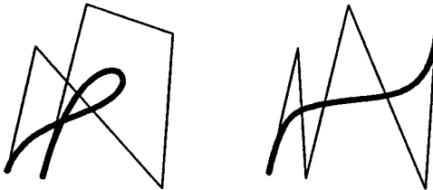
Figure 2: Two polygons (thin line) with associated Bézier curves (thick line)
